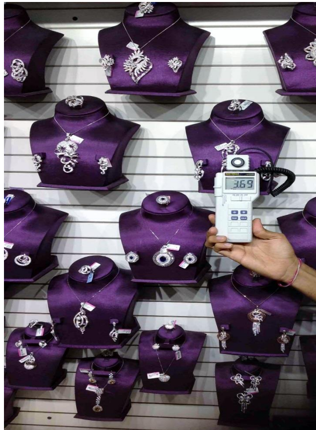
Brightness: 3.69K or 3690 LUX At the distance of 1.30m from the lamps
